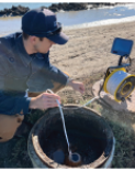
Valley Water staff evaluating a seawater intrusion monitoring well near south San Francisco Bay.
